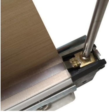
Figure 9. Screw element in place.
