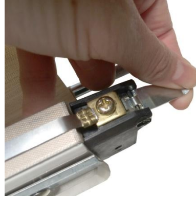
Figure 10. Lift latch on heating block to secure element in place.
