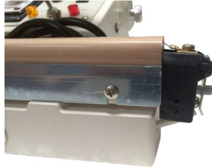
Figure 8. Remove heating element cover.
